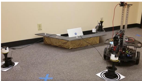
Figure 3. A Mock Lander equipped with the required parts for three antenna array units. Each antenna array unit consists of an antenna module (black) and a USB module (white). Unit 1 has already been deployed, unit 2 is being assembled, and unit 3 remains on the lander.
