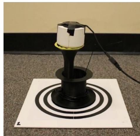
Figure 6. Fully assembled and deployed antenna unit. The black case is the antenna module. The white case is the USB module. The modules are connected via a magnetic micro USB.
