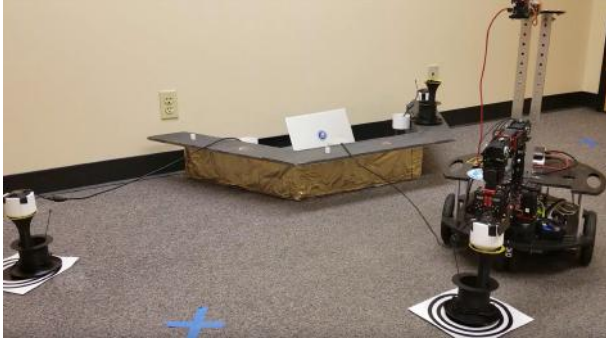
Figure 7. The Mock Lander equipped with the required parts for three antenna array units. The antenna modules are black, and the USB modules are white. Unit 1 has already been placed, unit 2 is being assembled, and unit 3 remains on the lander.
